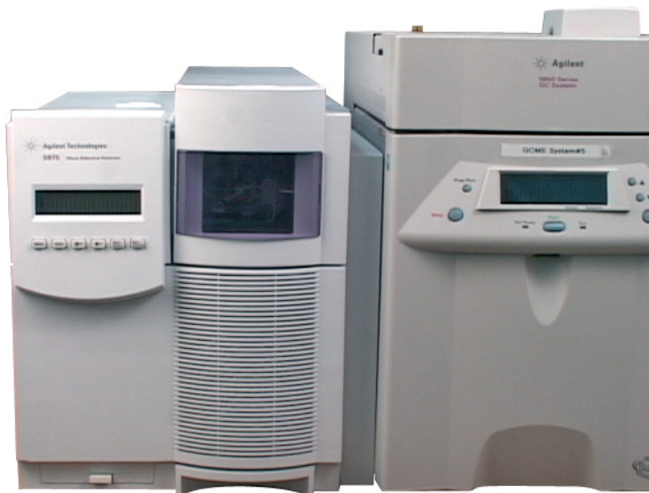
Figure 12 MSD and 6850 GC properly positioned
