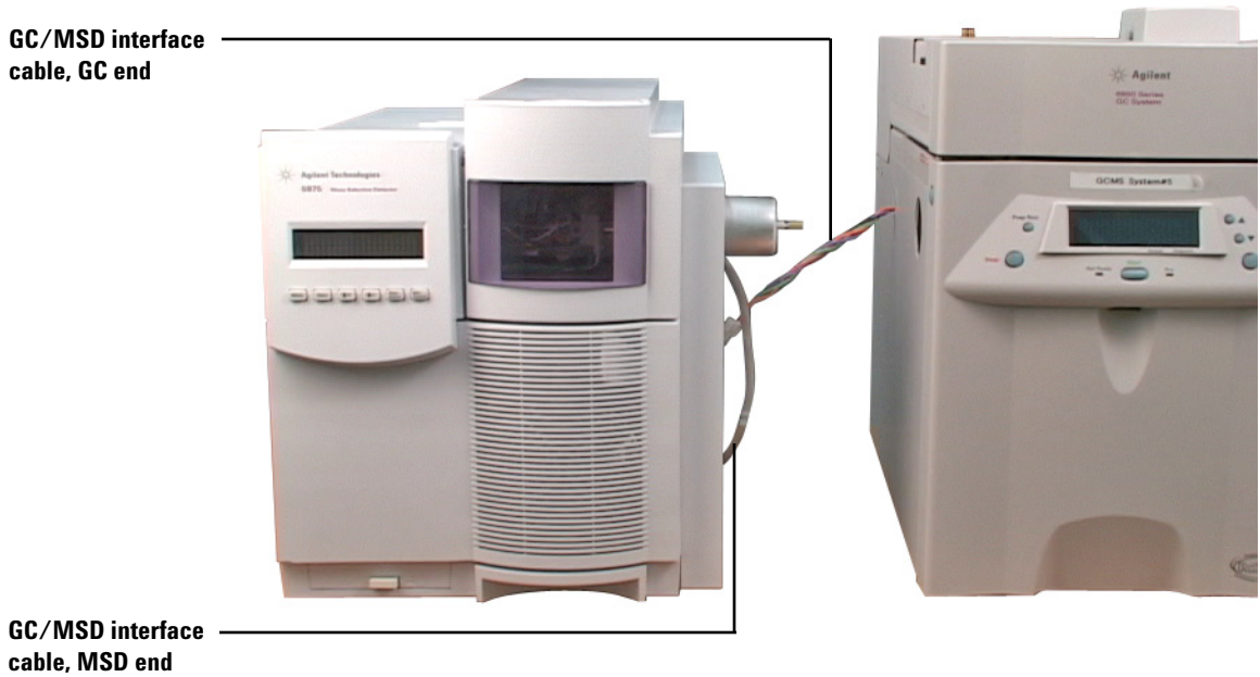
Figure 11 Interstitial panel installed, GC/MSD interface cable connected
